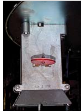
Latched Position Reflector Visible from Ground
