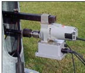
Portable motor mounted to pole (Option LD)
