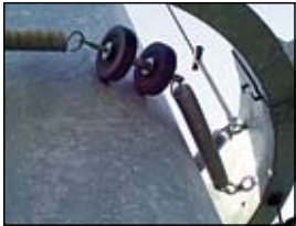
Detail view of the optional patented centering spring design (Option CS)
