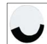
CL60x135 - Internal 60° Vert. x 135° Horiz. Lens Shielding
